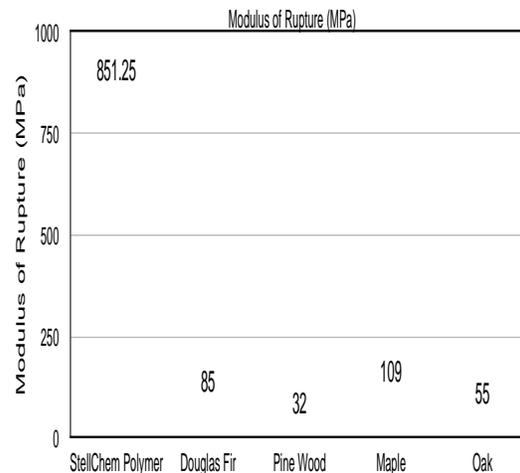
**Figure 2:** Comparison of modulus of rupture
